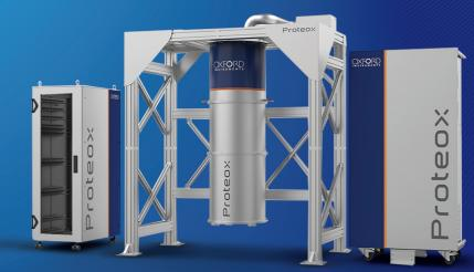
Lower electron temperatures with Oxford Instruments' coldest Proteox dilution refrigerator Oxford Instruments' coldest continuous operation Cryofree<sup>®</sup> dilution unit provides an ultra-low base temperature of < 5 mK and high cooling power of > 25 uW at 20 mK for optical access and Piezo positioners
